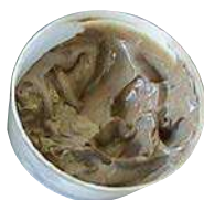
Used grease: colour turned greyish
