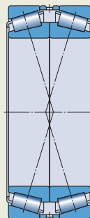
Matched bearings arranged face-to-face
