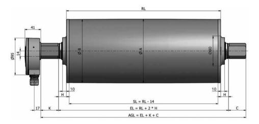
Drum motor with terminal box in aluminium
