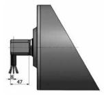
Cable slot 90° with threaded shaft
