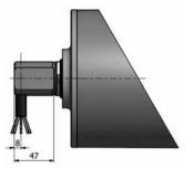
Cable slot 90° with threaded shaft
