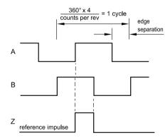
B leads A for clockwise rotation of magnetic actuator.
