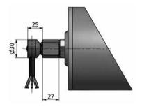
Elbow connector in stainless steel
