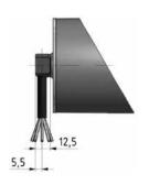
Cable slot 90° with threaded shaft
