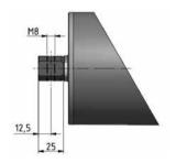
Cross-drilled and threaded shaft
