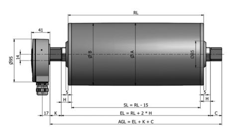
Drum motor with terminal box in aluminium
