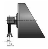
Cable slot 90° with threaded shaft
