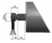
Elbow connector in stainless steel
