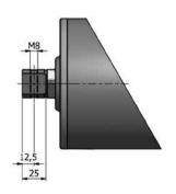
Cross-drilled and threaded shaft
