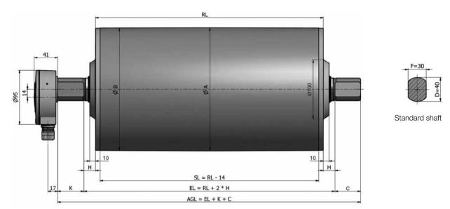
Drum motor with terminal box in aluminium
