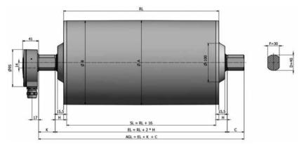
Drum motor standard version with terminal box in aluminium  $\leq$  4,0 kW
