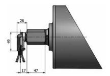
Elbow connector in aluminium
