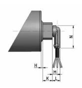
Elbow connector in aluminium
