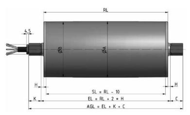
Drum motor with straight connector in stainless steel
