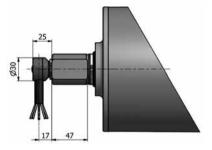
Elbow connector in stainless steel
