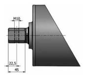
Cross-drilled and threaded shaft
