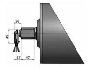
Elbow connector in aluminium
