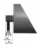
Cable slot 90° with threaded shaft
