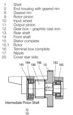
Pos. Description 20.1 Cover with labyrinth groove Cover front side 21 21.1 Cover with labyrinth groove 2 Dust lip seals on each side 24 26 Bearing Bearing 27 28 Bearing Bearing 29 30 Bearing 31 Bearing Retaining ring 32 37 Hexagon socket screw Hexagon socket screw 38 Hexagon socket screw 44 50 Waved spring washer 52 Magnetic oil plug 53 Distance washer 54 Distance washer Waved spring washer 66 70 Toothed washer 72 Taper grooved pin with internal thread 73 Set screw 75 Gasket 76 Gasket 77 Gasket
