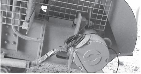
Compact and reliable drive unit using Motorized Pulley type 800H, 75kW at 3.15 m/sec.
