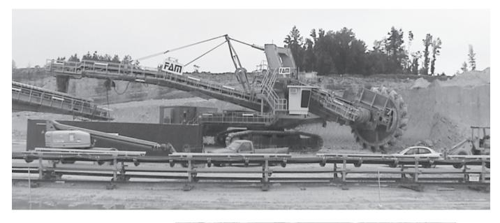
Excavator in a US cement application. Two Motorized Pulleys type 800H drive both the incoming & outgoing conveyors.
