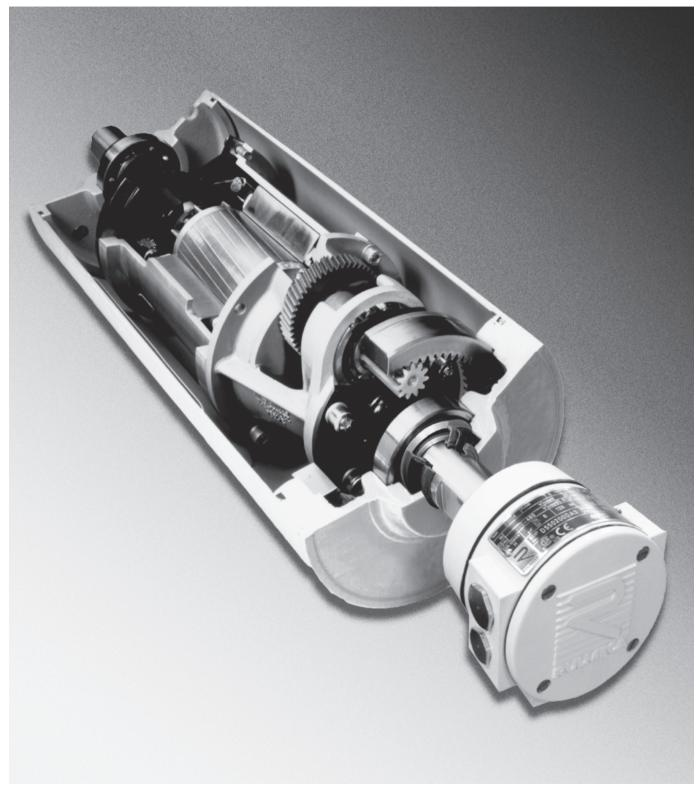
Sectioned model of Motorized Pulley type 220M.
