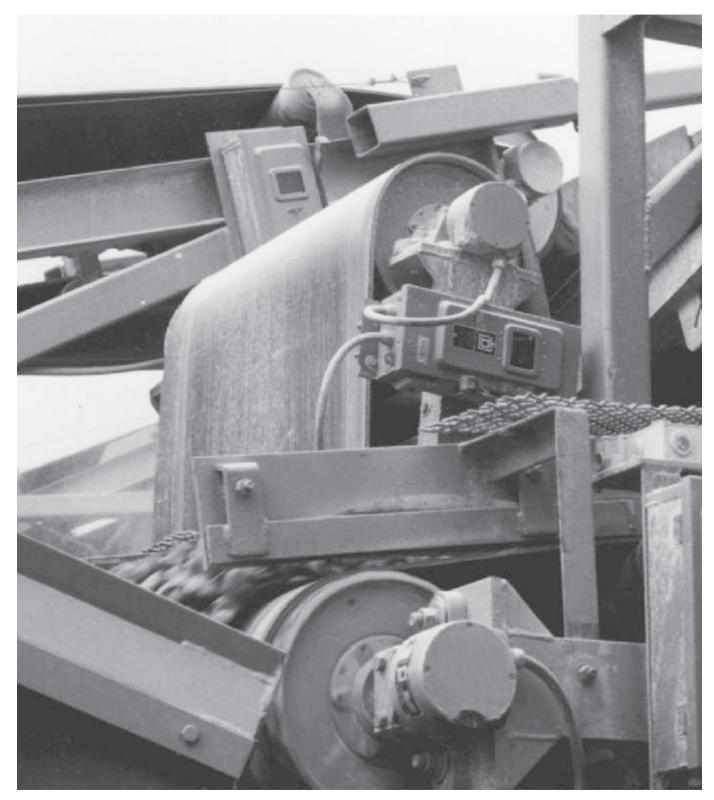
Rulmeca Motorized Pulleys in mobile Crushing & Screening. Features: Compact, reliable and requires NO maintenance!
