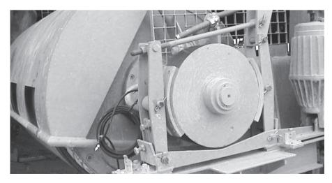
Both Motorized Pulleys are fitted with brake shaft for connection to external brakes.
