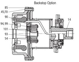
400M - 400H Electromagnetic Brake & Backstop Option
