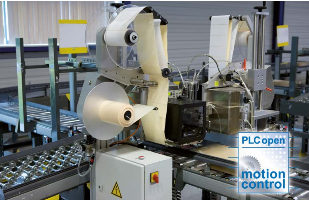
Labelling machine controlled by a L series PLC in combination with a Simple Motion module.
