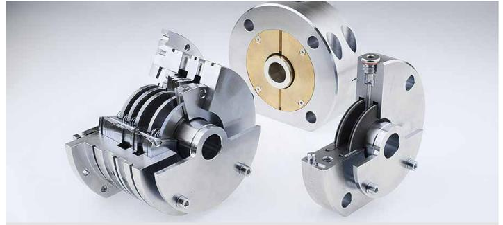
Carbon floating ring seals are supplied as maintenance-free compact labyrinth cartridge seals with low leakage. The floating self-adjusting sealing rings provide radial sealing on the shaft with a very small gap. The seal requires no additional lubrication, and it is designed for dry running. Besides pure gas, carbon floating ring seals are also suitable for ATEX applications, toxic media, media containing solids, flue gas, dust, powder, vapor, liquid mist, oil mist and penetrating oil.
